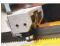
Saw blade guide made from carbide
